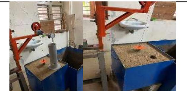
Fig. 6 Sand cone test laboratory setup
