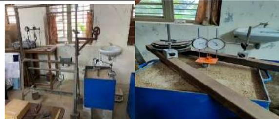
Fig.12 Pull-out test of Steel Pile
