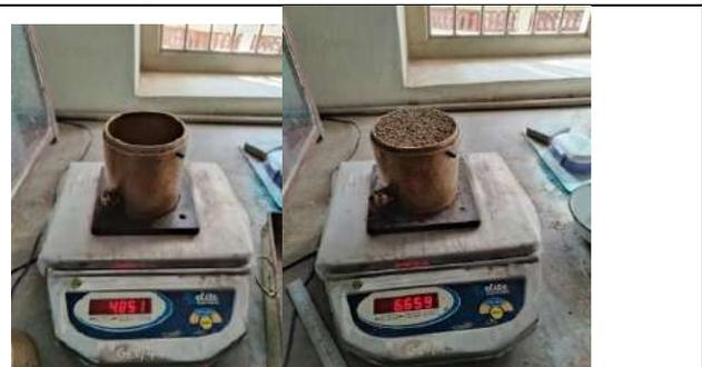
Fig. 4 Weighing mechanism in proctor test
