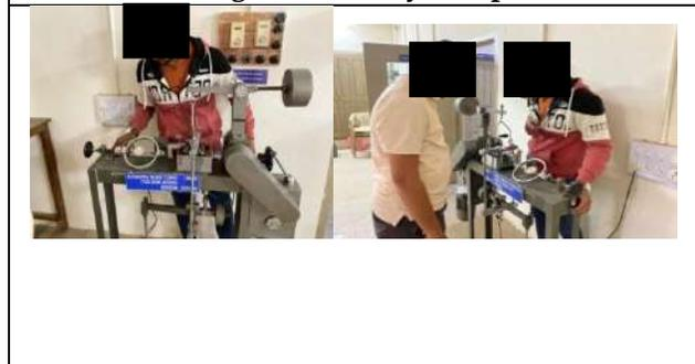
Fig. 3 Performing box shear test
