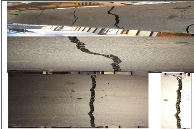
Figure 11 Rupture of the textile reinforcement fibre
