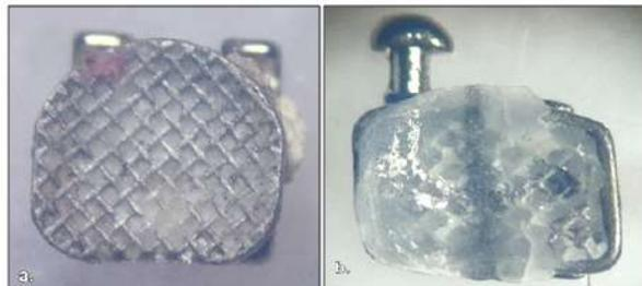
Figure 7 Scanning electron micrographs of the bracket base after debonding
