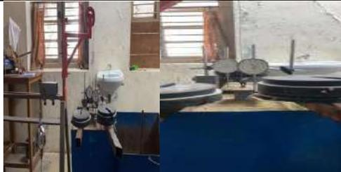
Fig.11 Pull-out test of Concrete Pile
